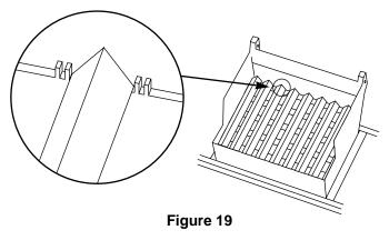
The open "U" of the cooking grates goes down. Set the cooking grates onto the ledges in the cooking box. Figure 20.
